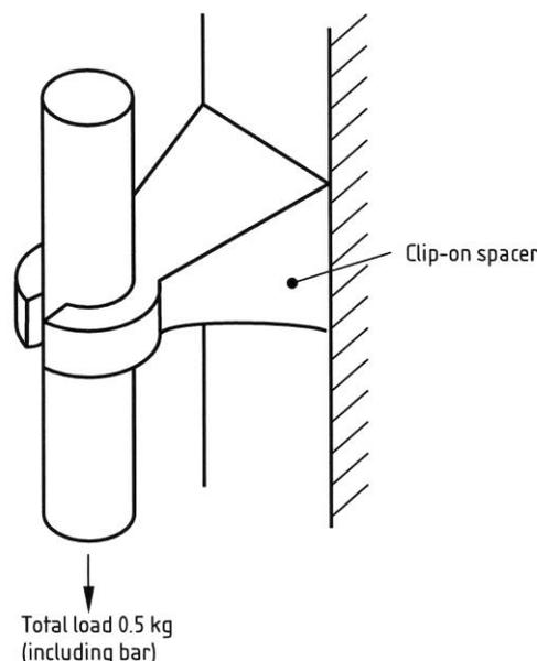
Figure 2. BS 7973-1:2001, Figure 2. Isometric view of the fixity test for clip-on spacers.
