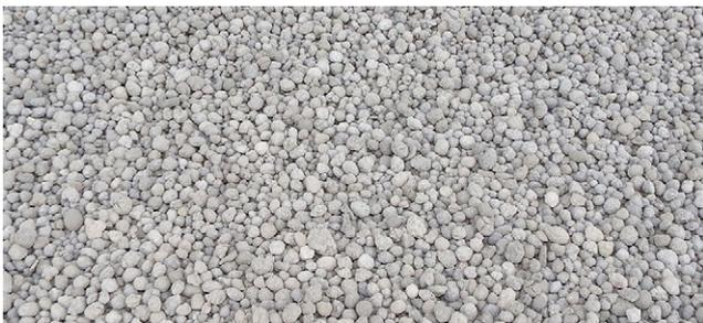
Figure 2. Example of carbon-negative aggregate
